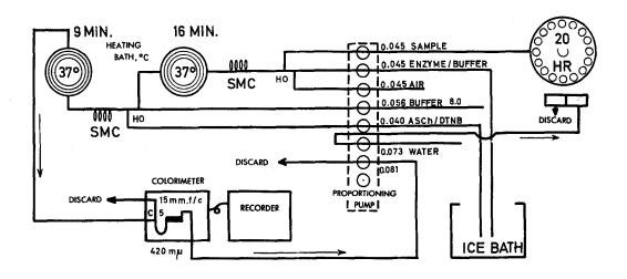
Figure 1. Flow diagram of the automated cholinesterase inhibition procedure 4) described by Voss and Geissbühler (4).
